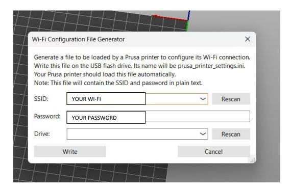
Click on Write, PrusaSlicer will confirm saving configuration file on to the USB drive, safely eject USB drive using eject icon.
