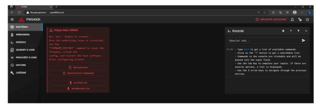
The error message of the clipper is normal when starting the printer for the first time, using the button to restart the firmware, a correct window will appear offering to turn on the printer.
