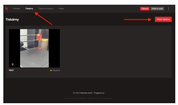
Open the Printers panel. Here is the Add Printer button-Assigning the printer to your account is done using the same procedure
